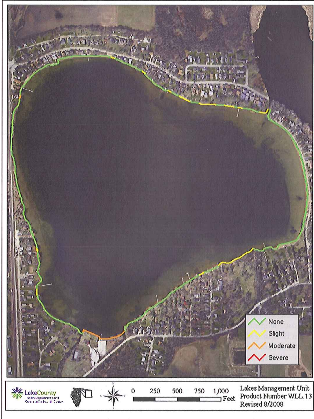
Figure 13. Shoreline erosion on West Loon Lake, 2008
