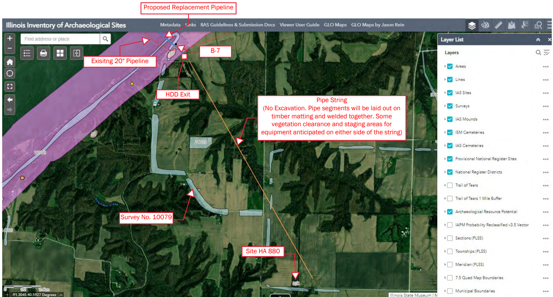
Figure 7: Aerial Map showing approximate location of the pipe segment stringing and welding in relation to previously recorded archaeological survey areas, archaeological resource potential areas, archaeological sites, cemeteries, mounds and NRHP listed and eligible resources. No excavations will occur, but activities such as laying of timber mats for access and staging areas for unloading pipe segments, pipe welding and coating, and layout of padded wooden skids to support pipes etc. are expected.
