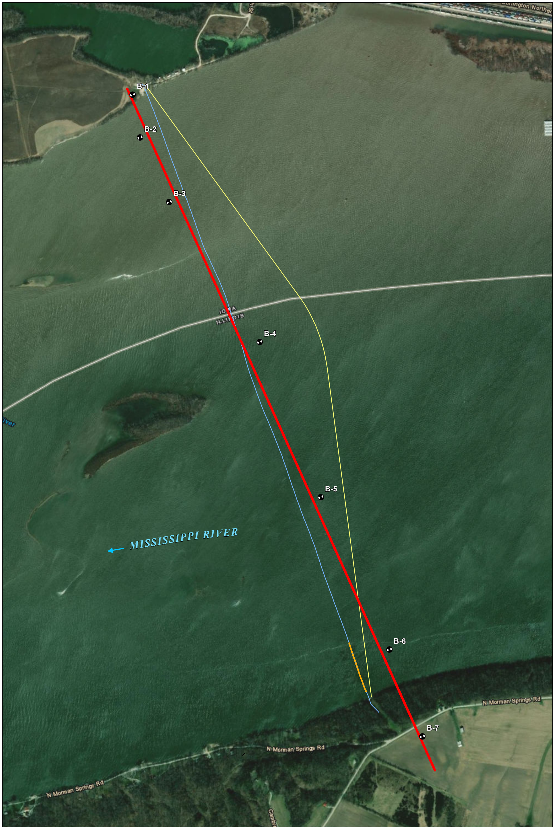
Figure 2. Aerial Map of Site with Impact Areas for the BP One Pipeline Company LLC's, Mississippi River Geotechnical Boring/HDD Pipe Replacement and Possible Emergent Repairs. Hancock County, Illinois.
