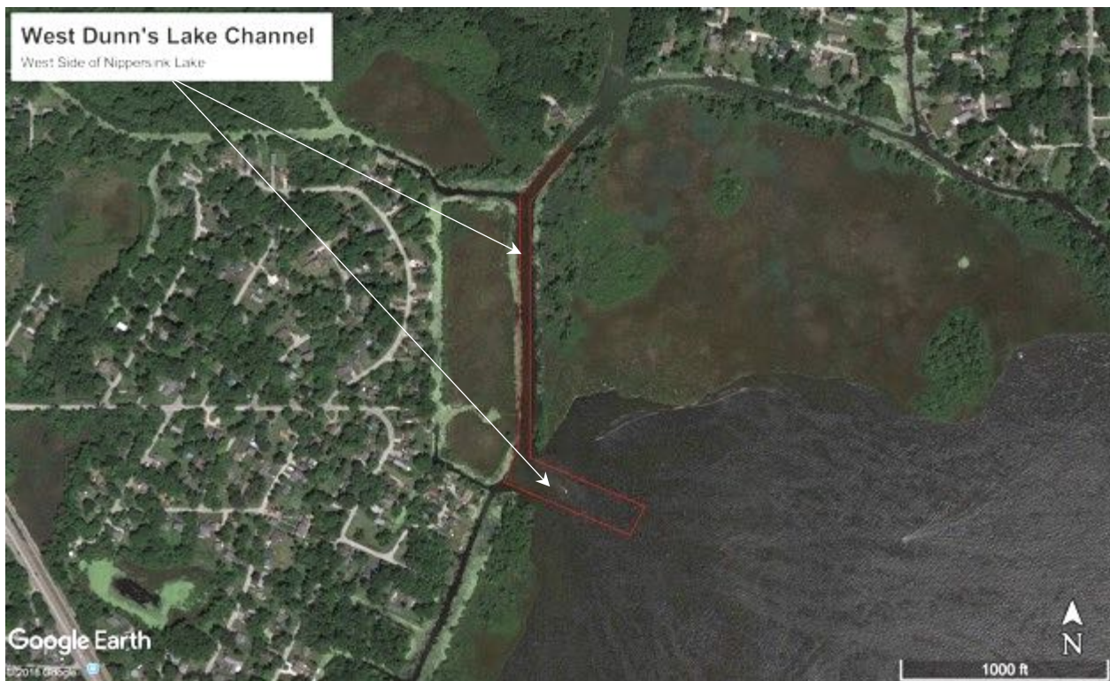
Figure 15. West Dunn's Lake Channel on Nippersink Lake (AN-18 Hydraulic Dredging - 7.6 ac)
